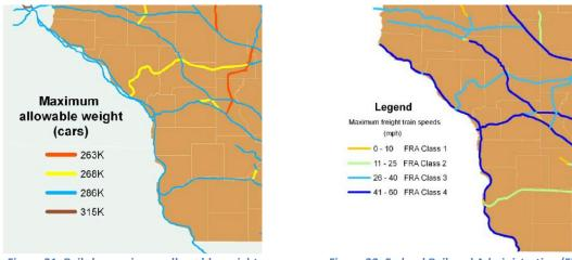
Figure 31. Rails by maximum allowable weight
