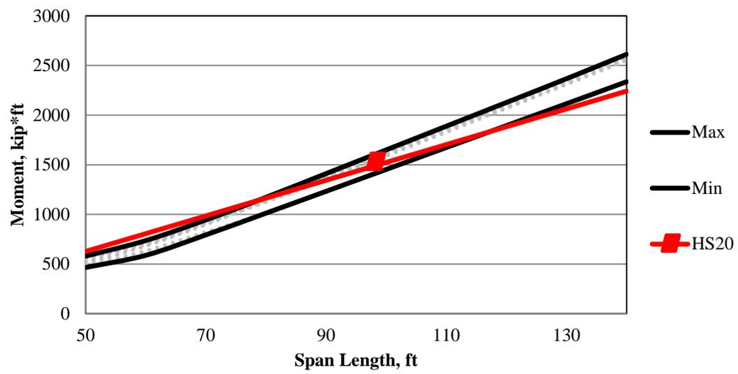
Figure 6-35: Moment envelope of the six-axle vehicles compared to the HS20
