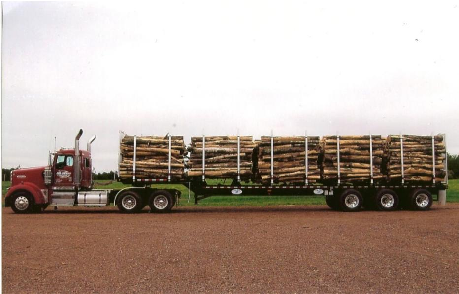
**Figure 6-2: Standard Six-axle Tractor Trailer(Great Lakes Timber Professionals Association, 2009)**
