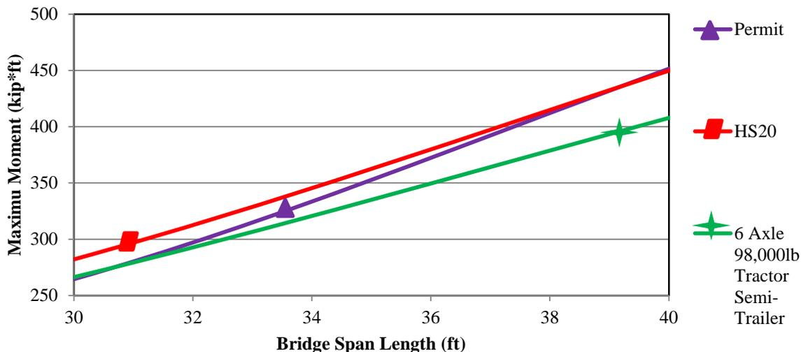
Figure 6-40: lower bound limits for TSW Six-axle 98,000-lb Tractor Semi-Trailer
