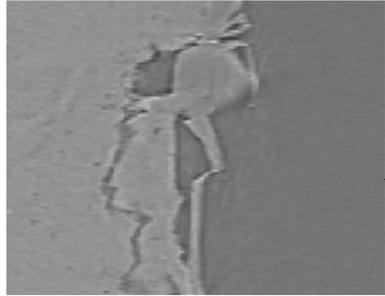
Propagating crack and angular pore connected to aggregate surface
