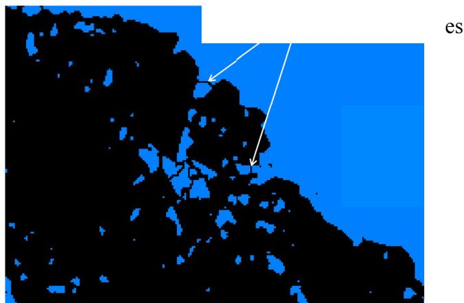
**Figure 3.28: Lines from “binseparate” command created to split pores from background**
