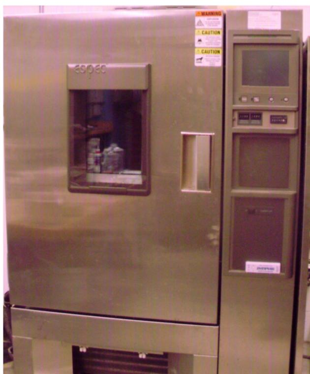
**Figure 3.4: Freezing and thawing chamber used in this study**
