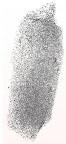
(b) 3D volume rendering of pores within the aggregate
