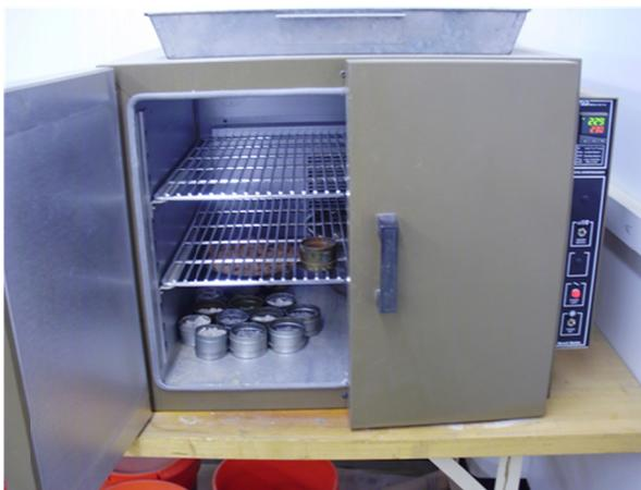
**Figure 3.5: Drying oven used in this study to dry aggregates**
