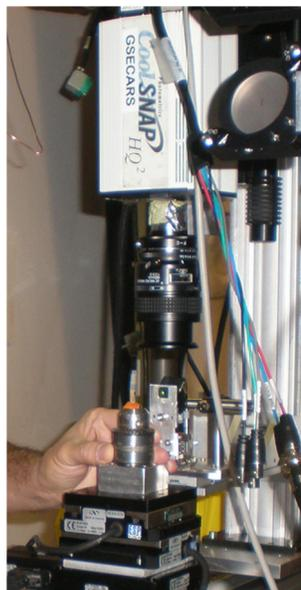
**Figure 3.13: Sample on rotation stage, scintillator, mirror and CCD system**
