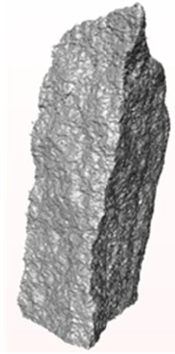
(a) 3D surface generation of an aggregate
