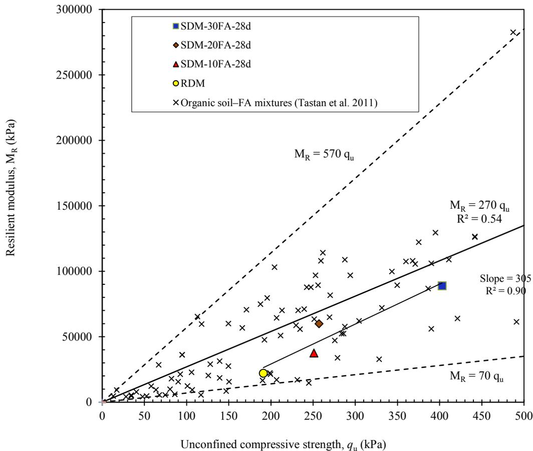
Fig. 2.12.  $M_r$  versus  $q_u$  for RDM and SDM specimens
