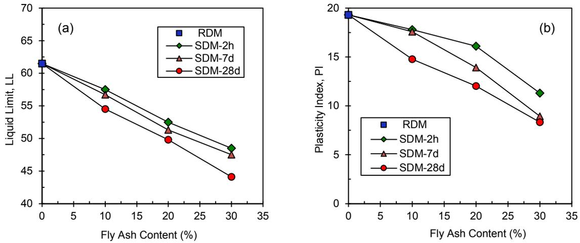
Fig. 2.2. LL and PI versus FA content for RDM and SDM specimens
