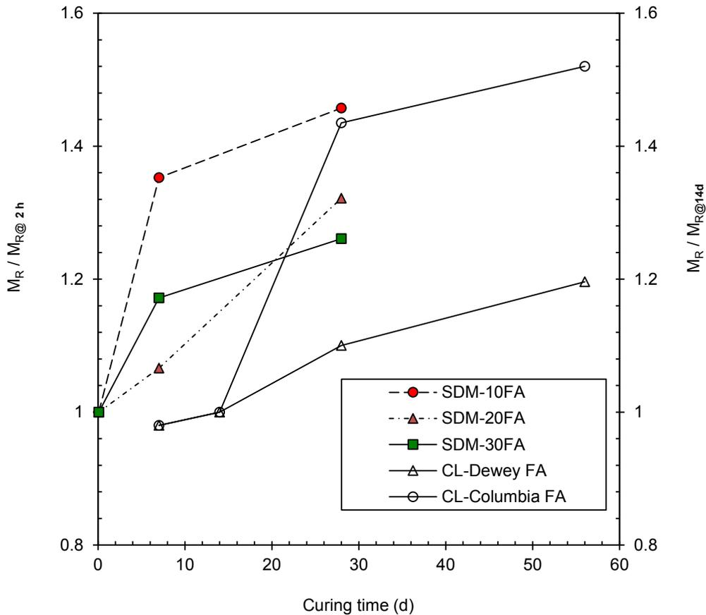
Fig. 2.10. Effect of curing time on  $M_R$
