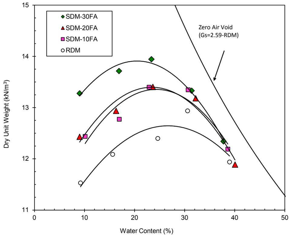
Fig. 2.4. Compaction curves of the RDM and RDM-FA mixtures
