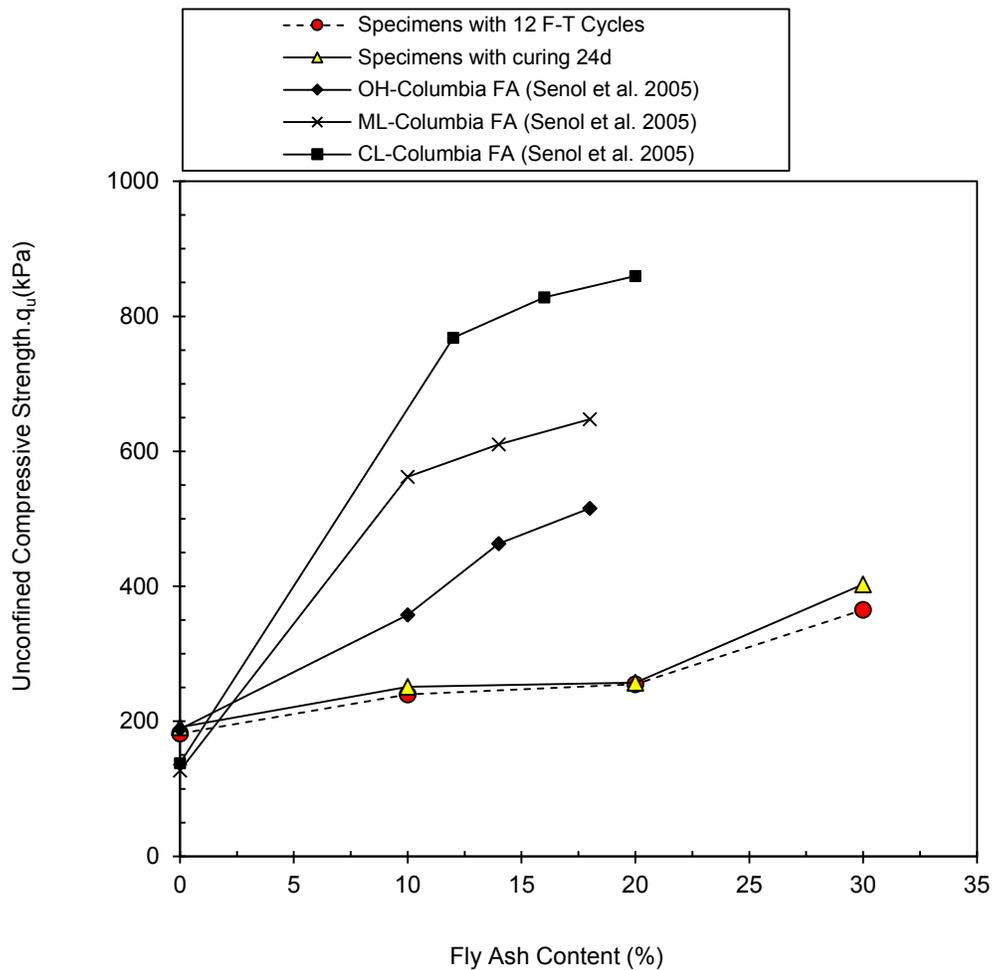
Fig. 2.7. Variation of unconfined compressive strength of SDM specimens with FA content and freeze-thaw (F-T) cycles
