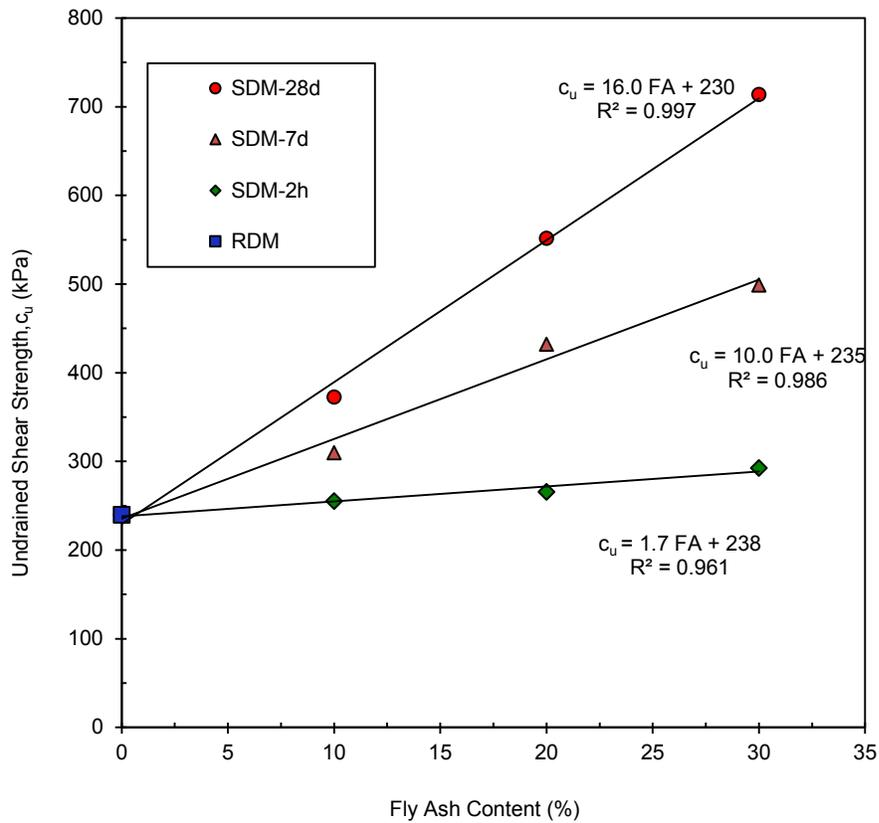
Fig. 2.6. Variation of undrained shear strength with FA content and curing time
