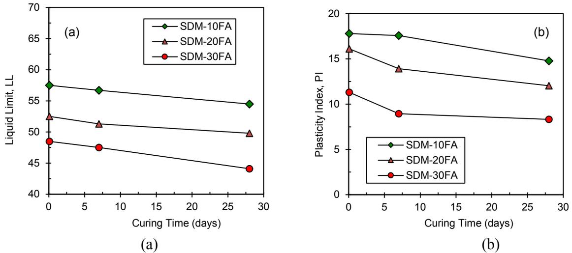
Fig. 2.3. LL and PI versus curing time for RDM and SDM specimens
