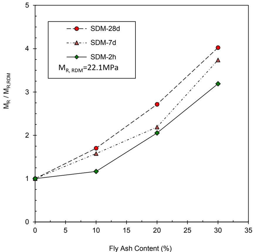
Fig. 2.9. Variation of  $M_R / M_{R,RDM}$  with FA content and curing time
