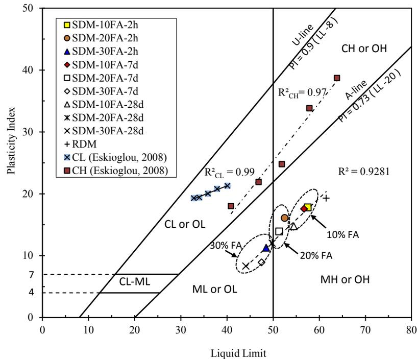
Fig. 2.1. Atterberg limits for RDM and SDM specimens
