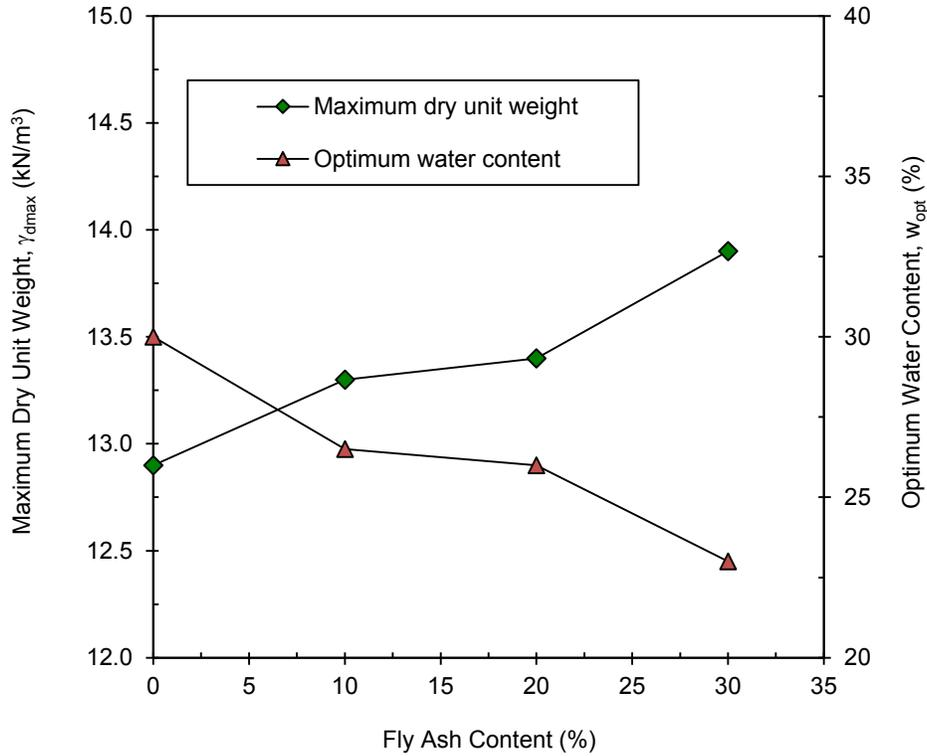
Fig. 2.5. Variation of optimum water content and maximum dry unit weight with FA content
