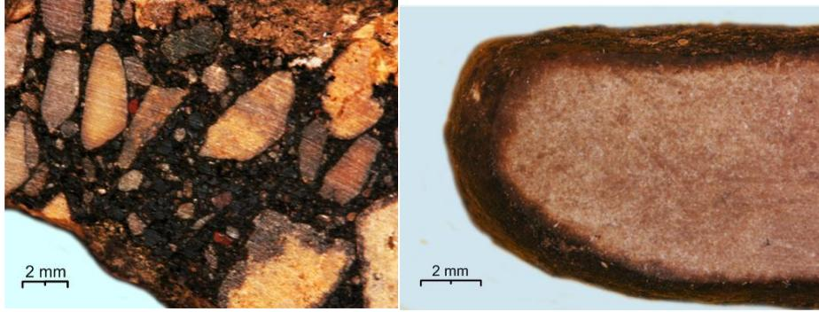
Figure 2.1 RPM aggregates coated with asphalt binders
