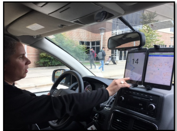
Andi Bill, UW TOPS Lab traffic safety manager, demonstrated how a Dedicated Short-Range Communication unit within a vehicle broadcasts the signal phasing and timing information.
