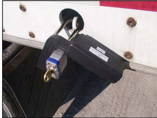
Figure 5: E-Seal Attached to Freight Trailer (5)
