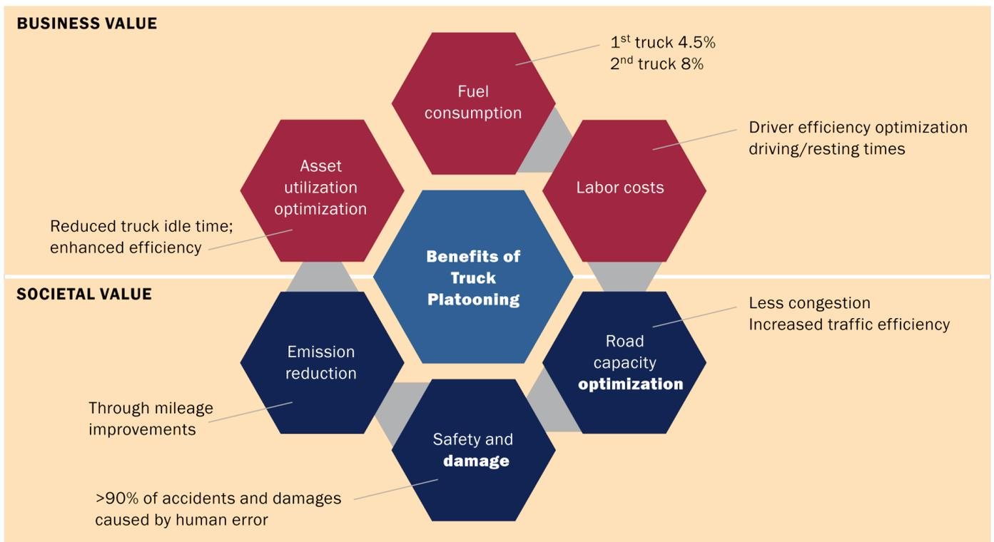
Graphic based on diagram by TNO in "Truck Platooning - Driving the Future of Transportation."
